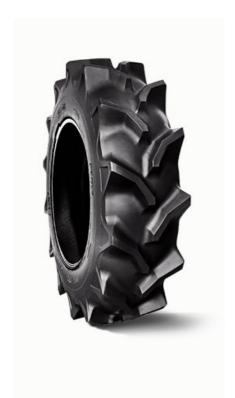
**Description** TR 173 is a tractor tire suitable for wet conditions and
