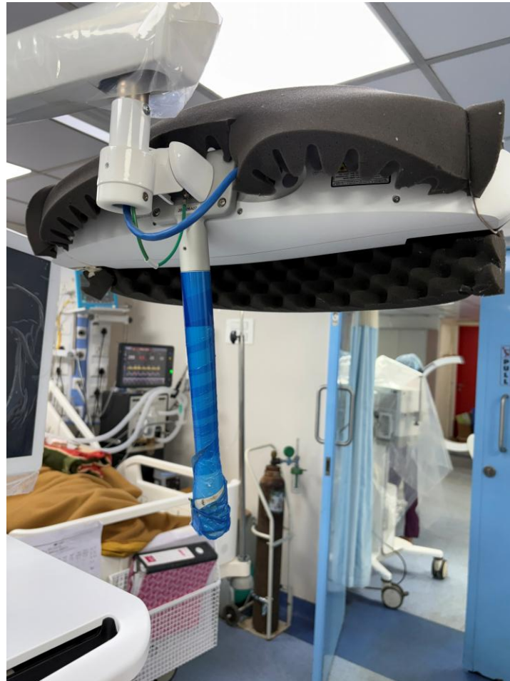
Optical Tracking Sensor System of CUVIS Joints - Tracks patient anatomy and instrument positions in real-time and ensures optimal alignment and accurate imitation of the planned cuts.
