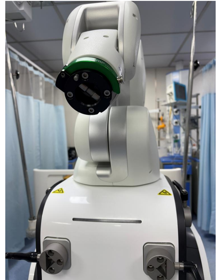
Robotic arm of the CUVIS Joints - Performs automatic and precise bone cutting based on the surgical plan.
