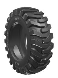
SKID POWER PLUS has been designed for skid steers in construction applications. Its wider lugs provide excellent traction as well as enhanced self-cleaning properties. The tire features an extra deep tread along with enhanced sidewall protection providing excellent cut-and-chip resistance and outstanding durability. SKID POWER PLUS is the ideal tire for loose surfaces. The wide contact area provides excellent stability during operations.
